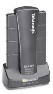
► The Tektronix BPA105 Bluetooth Protocol Analyzer consists of version 2.4 Analysis Software and the air probe which houses the Bluetooth V1.1 compliant baseband controller and radio.
